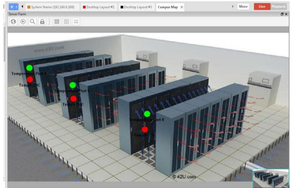
Custom user desktop—in this instance the red icons represent PDU's where the load is nearing maximum levels
