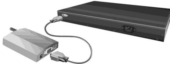
Figure 3-17 Connect GSM modem to interSeptor Pro
