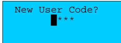
Type the new operator code for the ZonePod speech dialler and press “ENT”. This will be the code that you will have to type in order to access the menu locally from the main screen.
