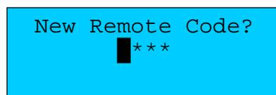
Type the new remote access code for the ZonePod speech dialler and press “ENT”. This will be the required code to dial into the unit remotely / access the unit during alarm calls.
