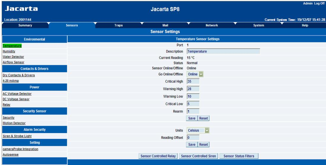
The sensors highlighted in green indicate that they are currently connected to the unit. In this case there is a temperature sensor connected and so Temperature is highlighted in green in the menu.
